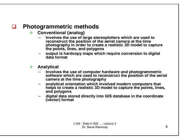
This third data acquisition method is through the use of aerial photos. There are two methods used to extract data from aerial photos which are analog and analytical methods. This slide gives a brief, yet self explanatory description of each method.
