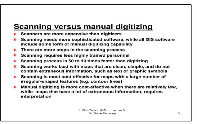
This slide compares scanning versus manual digitizing. Scanning is the conversion of hardcopy data into pixel data sets. Which is better, digitizing or scanning?
