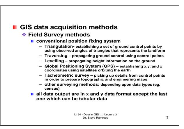
The first data acquisition method is through field survey methods. There are various field survey methods for the various professions. Typically, the most common methods are through the Geomatics field where surveying instruments are used to capture data from the field. Data such as angles, distances, coordinates, and such like are typical data sets captured from the Geomatics field which are processed to generate the coordinates of points lines and area features.
