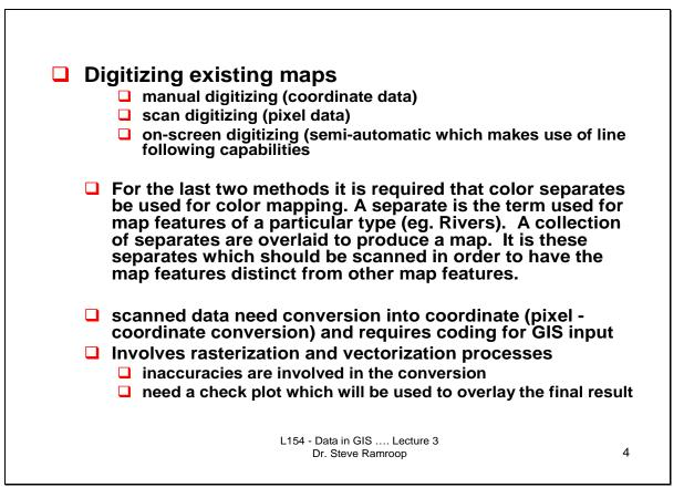
The next method of acquiring data is a method called digitizing. This is one of the common methods used to capture data from hardcopy maps into digital computer format. Three methods are identified. Manual digitizing is the use of a digitizing table which is connected to a computer that utilizes the digitizing table through its application software. Hardcopy maps are placed onto the table, and then ground coordinates are registered using the table and the application software. On
