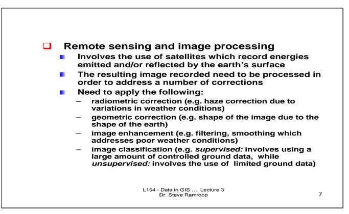
The fourth data acquisition method is data obtained from the satellites. The data sets from satellites are images which require post processing. Four of the post processing procedures are identified on this slide. Note that when data is taken out from satellites the spherical nature of the earth's surface introduces various errors associated with the image, and in addition other corrections need to be applied.
